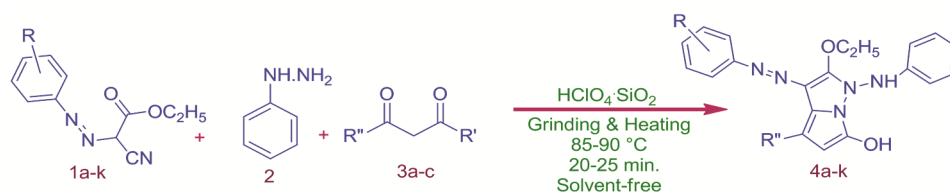
Scheme 1 — Multicomponent solvent-free synthesis of pyrrolo[1,2- b ]pyrazole derivatives 4a-k using \text{HClO}_4 \cdot \text{SiO}_2 as a supported catalyst
