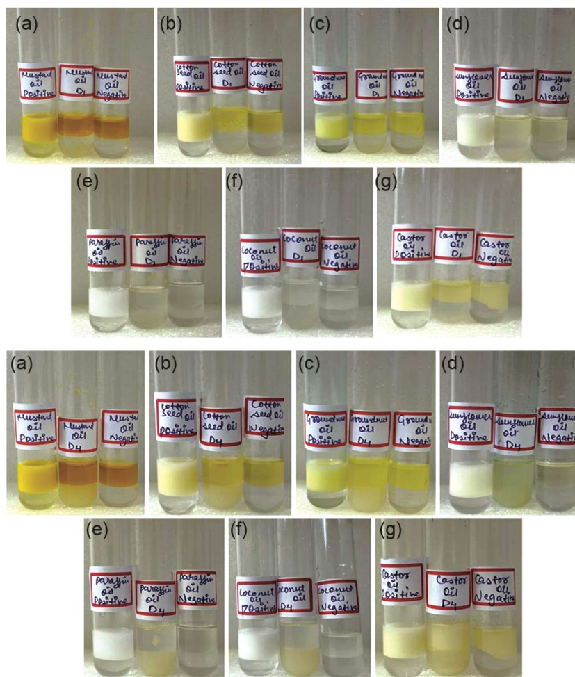
Fig. 2 — Emulsification activity of (a) Halomonas sp. DU-15-9-1; and (b) Salinicoccus roseus S-5-9-3 isolates by using different oils: A=Mustard oil, B=Cottonseed oil, C=Groundnut oil, D=Sunflower oil, E=Paraffin oil, F=Coconut oil, G=Castor oil.
